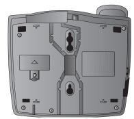
2 Remove the battery compartment screw with a small Phillips head screwdriver.
