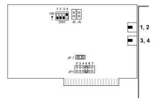
The following diagram illustrates the D/4xD board. The location of the relevant jumpers and switches on the D/42D-SX and D/42D-SL boards are approximately the same as on the D/4xD board.
