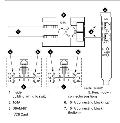
Figure 4-2. Connecting IVC6 Cards Using 104A Connecting Blocks
