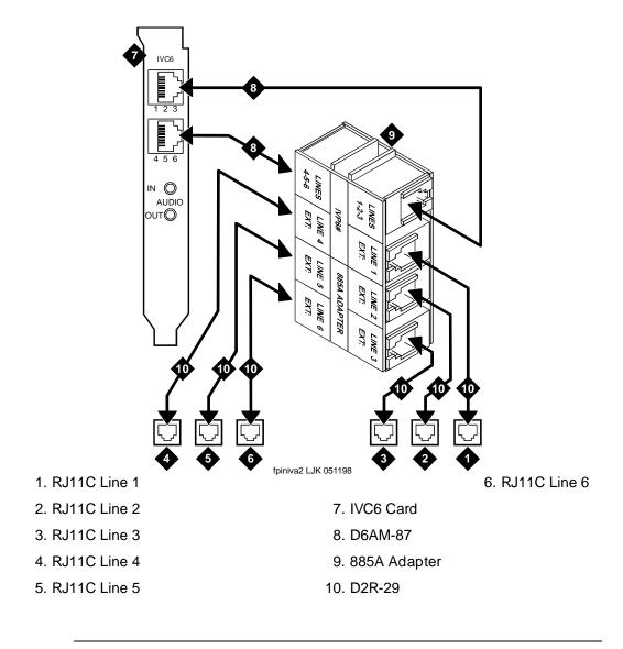
Figure 4-1. Connecting IVC6 Cards Using an 885A Adapter
