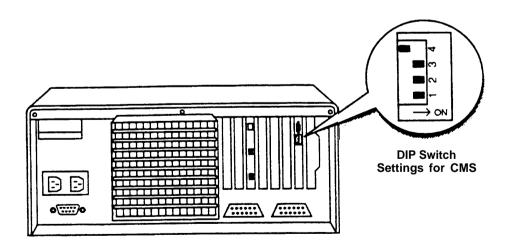
Figure 2-2. VDC 600 DIP Switch Locations and Settings
