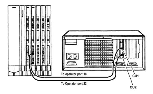
Figure 2-3. Connecting CU1 and CU2 to the MERLIN LEGEND Control Unit
