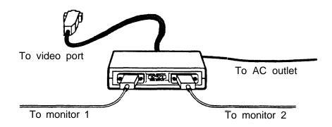
Figure 2-5. Connecting a View-Only Monitor
