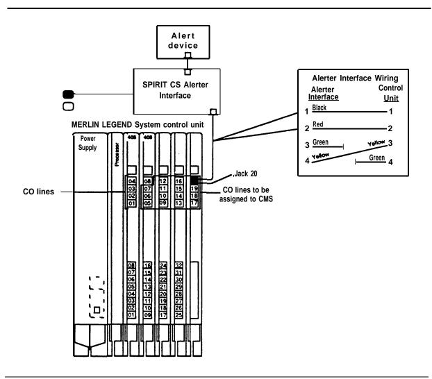
Figure 2-1. CMS External Alert Connection
