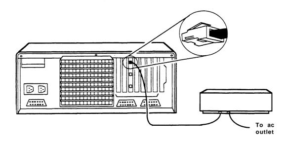
Figure 2-4. Connecting the VAU to the CMS PC
