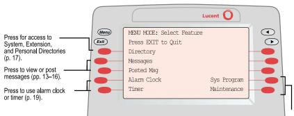
If your console is set up for system programming and maintenance, Sys Program and Maintenance are shown on the right side of the Menu screen. If you have not been trained or are not familiar with these features, see your System Manager.
