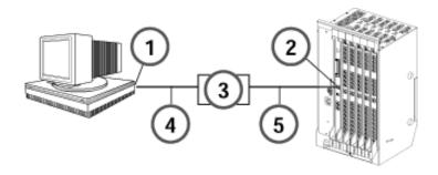
Figure 3-2. Direct Connection, PC Less Than 50 Feet Away
