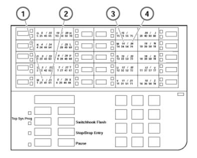
Figure 2-7. MLX-20L System Programming Console Overlay
