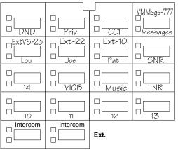
Intercom Autodialer is programmed with Intercom Auto Dial and Manual Signaling buttons for 31 extensions; the order of extensions has been changed to begin with extension 11 on the top left button. The user's 18-button telephone has 5 individual lines assigned; the other 11 buttons are used for Intercom Auto Dialing and dial-code features.
