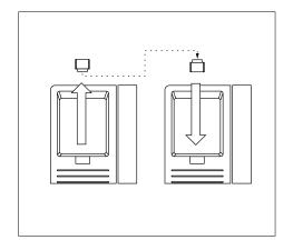
Holding the wall mount with the wide edge down, mount it on the wall plate, aligning the keyholes on the base of the wall mount to the wall plate. For proper mounting, the wall plate must be a Lucent Technologies 630B connecting block.
