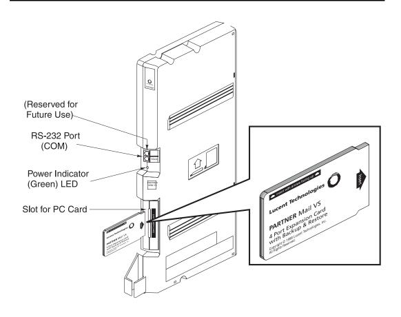
Figure 2-2. Installing the PC Card
