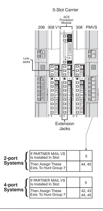
Figure D-7. Dial Plan for Systems with Fax Tone Detect and a Voice Messaging System Module
