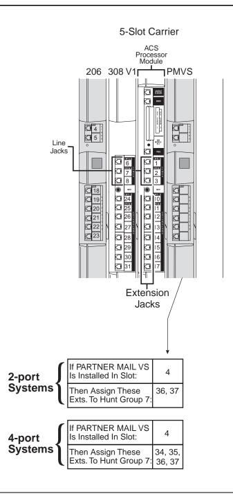
Figure D-6. Dial Plan for Systems with Fax Tone Detect and a Voice Messaging System Module
