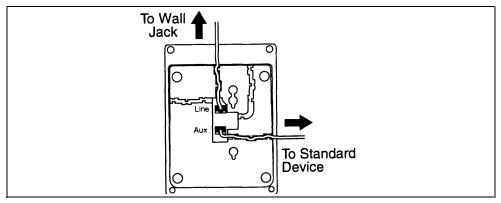
**Figure 2. Combination Extension Using Direct Connection**
