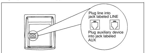
Figure C-4. Combination Extension Using Direct Connection
