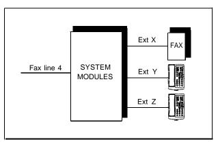
Figure 4-5. Fax Machine with its Own Line
