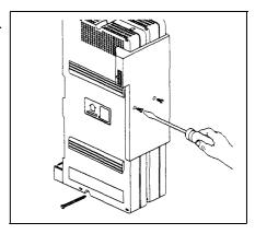
2 Slide off the module furthest from the wall—without detaching the line and phone cords. If you are replacing the module furthest from the wall, go to Step 4; if you are replacing the one closest to the wall, go to Step 3.
