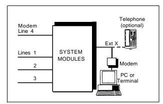
Figure 4-9. Send and Receive Modem
