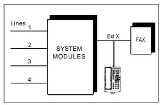
Figure 4-7. Fax and Telephone Combination
