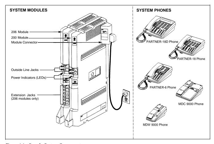
Figure 1-1. Sample System Components
