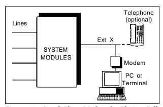
Figure 4-8. Stand-Alone Modem for Placing Calls Only
