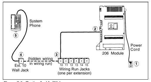
Figure C-2. Testing Inside Wiring
