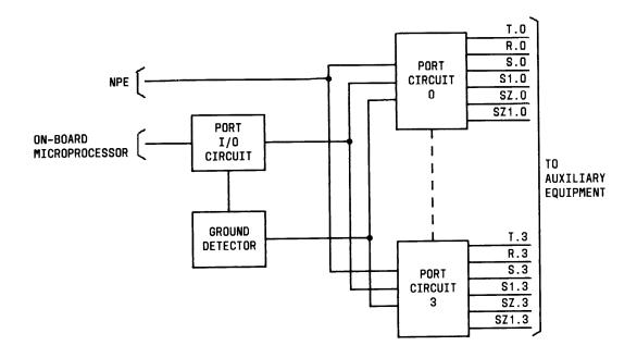
Figure 3-9. Auxiliary Trunk (TN763) Unique Circuitry
