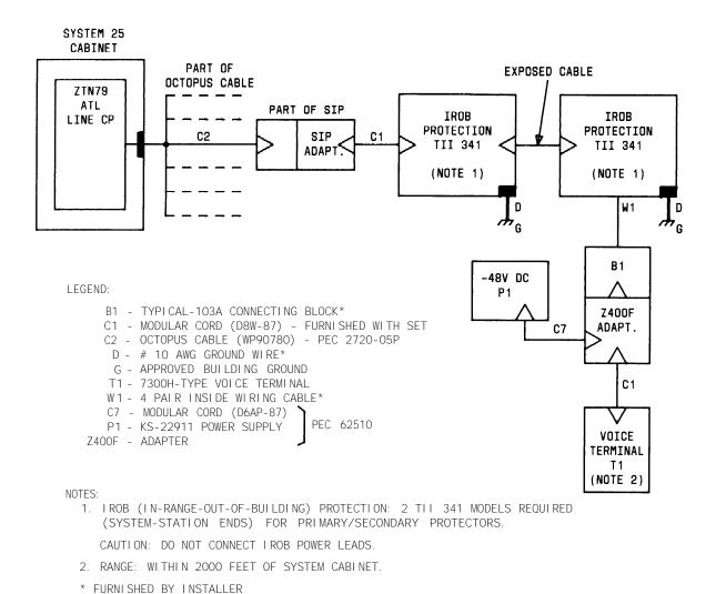
Figure 4-30. Out-of-Building 7300H Series Multiline Voice Terminal Connections
