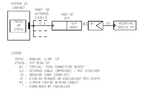
Figure 2-19. External Alert Connections
