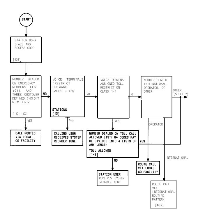
Figure 2-8. Automatic Route Selection Flow Chart (Sheet 1 of 2)
