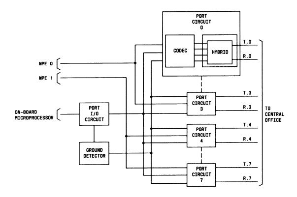
Figure 3-12. Ground Start Trunk (ZTN76) Unique Circuitry
