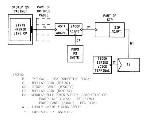
Figure 4-32. Stand-Alone Remotely Powered Voice Terminal Connections
