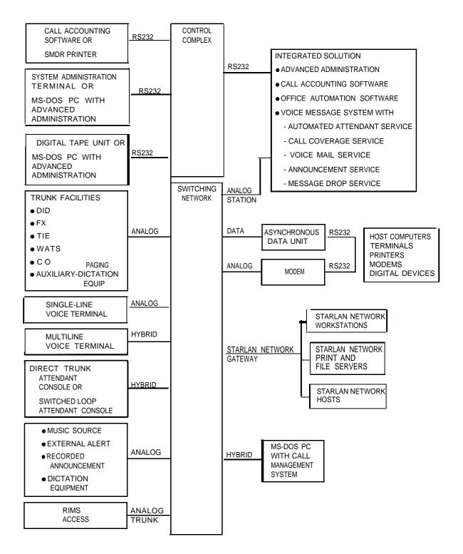
Figure 1-1. System 25 Block Diagram
