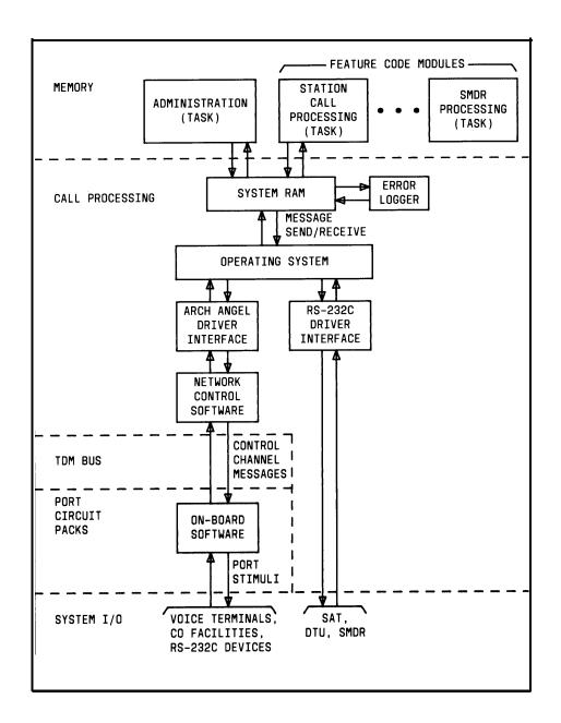
Figure 3-21. System Software Partitioning
