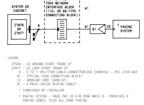
Figure 2-29. Paging Equipment Connections Using CO Trunk Ports (FCC Registered)
