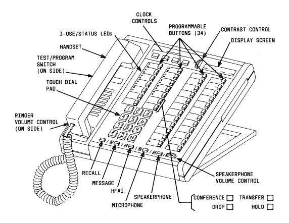
Figure 4-13. 7305H04C Voice Terminal (BIS With Display)
