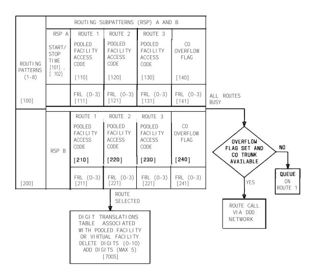
Figure 2-9. Automatic Route Selection Routing Pattern
