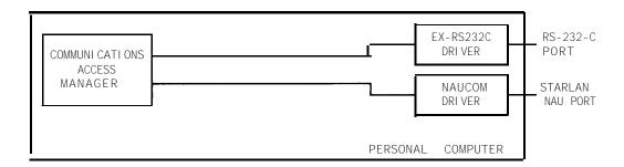
Figure 2-13. Communications Access Manager Architecture
