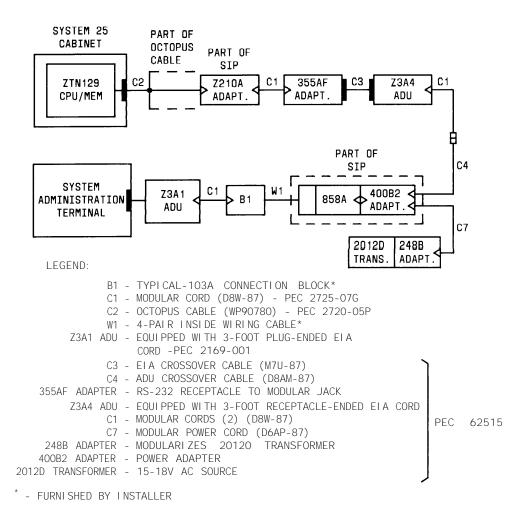
Figure 2-51. SAT On-Premises Direct Connections (Greater Than 50 Feet From System Cabinet or Nonsharing Same AC Outlet)
