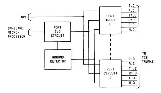
Figure 3-15. Tie Trunk (TN760B) Unique Circuitry
