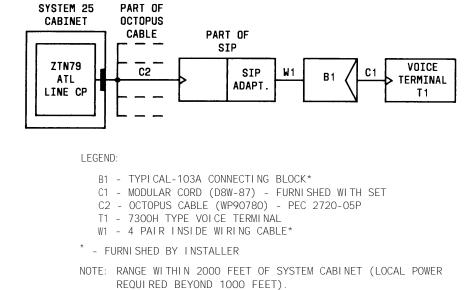
Figure 4-29. On-Premises 7300H Series Multiline Voice Terminal Connections
