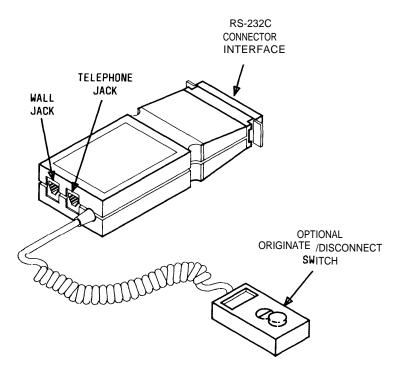
Figure 4-22. Asynchronous Data Unit (ADU)
