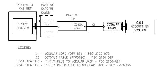
Figure 2-11. Call Accounting System—On-Premises Direct Connections (Sharing Same AC Outlet)
