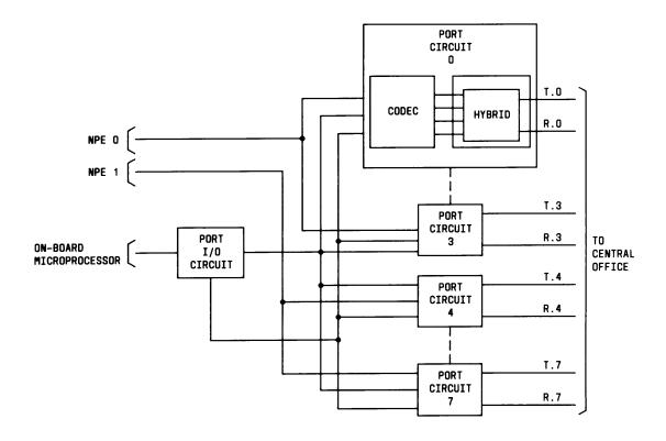
Figure 3-13. Loop Start Trunk (ZTN77) Unique Circuitry
