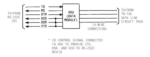
Figure 2-14. Asynchronous Data Unit Interface Signals
