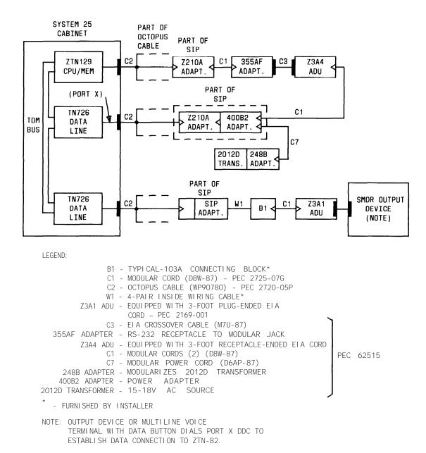
Figure 2-46. SMDR Output Equipment—On-Premises Switched Connections
