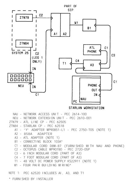
Figure 2-40. STARLAN NETWORK Connection to System 25 (With ATL-Type Telephone)
