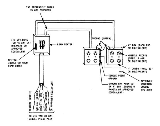
Figure 6-3. AC Power Distribution - Multiple Cabinet System
