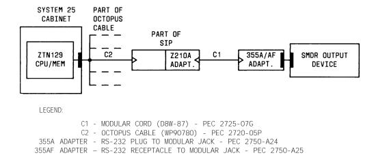
Figure 2-44. SMDR Output Equipment—On-Premises Direct Connections (Sharing Same AC Outlet)
