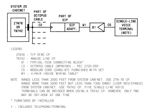
Figure 4-26. On-Premises Single-Line Voice Terminal Connections
