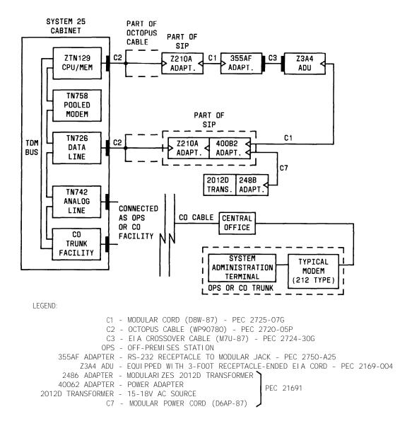
Figure 2-54. SAT Off-Premises Switched Connections
