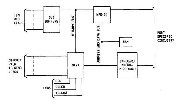
Figure 3-6. Port Circuit Pack Common Circuitry
