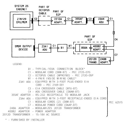
Figure 2-45. SMDR Output Equipment—On-Premises Direct Connections (Greater Than 50 Feet From System Cabinet or Nonsharing Same AC Outlet)
