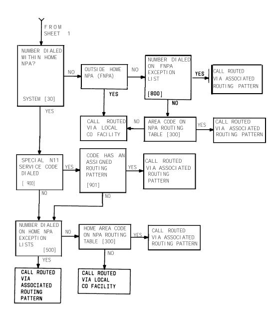
Figure 2-8. Automatic Route Selection Flow Chart (Sheet 2 of 2)
