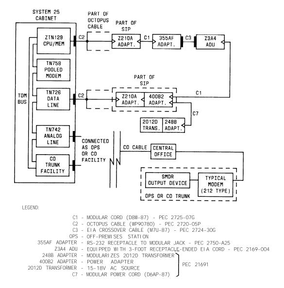
Figure 2-48. SMDR Output Equipment—Off-Premises Switched Connections
