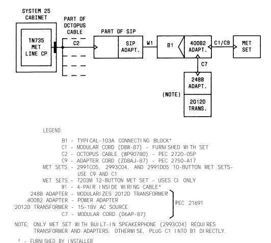
Figure 4-31. MET Set Connections
