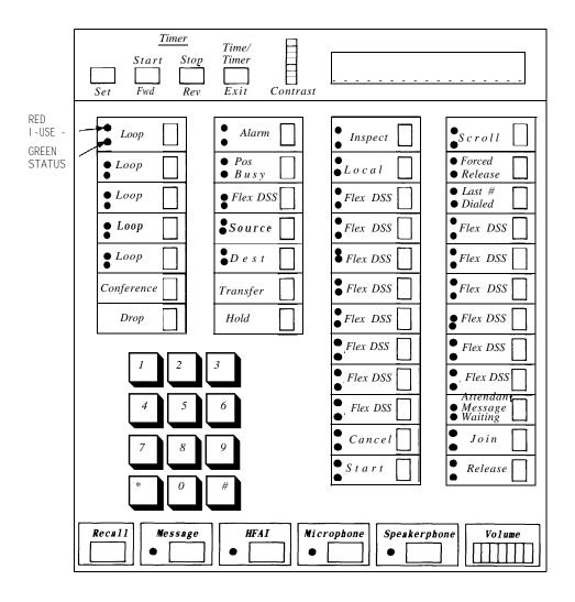
Figure 2-4. Buttons and Display of BIS-34D
