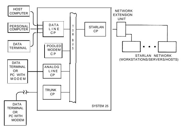
Figure 2-38. STARLAN NETWORK and System 25 Configuration
