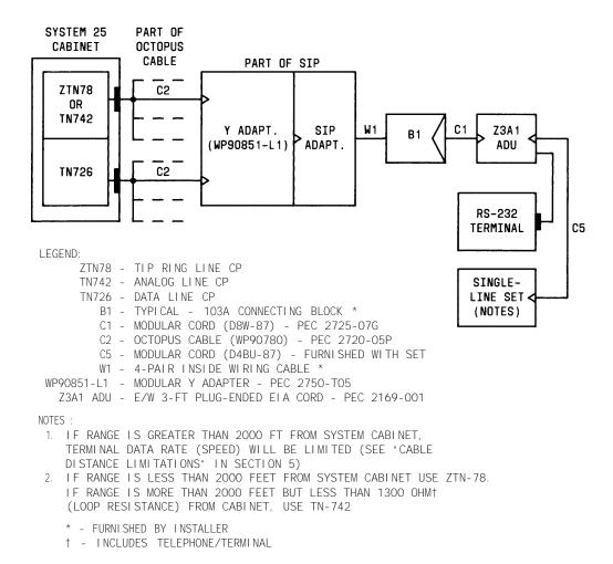
Figure 4-33. Typical ADU Connections—Supporting Data Terminal and Single-Line Voice Terminal
