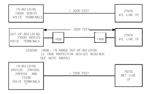
\* MODEL 2993CO4 (MET EQUIPPED WITH BIS) REQUIRES A 2012D POWER UNIT (15 - 18V AC)
