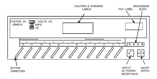
Figure 4-2. System Cabinet (J58901A)—Rear View
