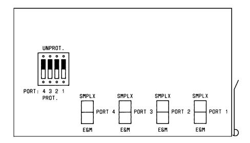
Figure 3-16. Tie Trunk (TN760B) Circuit Pack Option Switches
