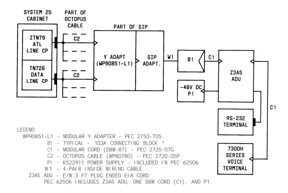
Figure 4-34. Typical ADU Connections—Supporting Data Terminal and 7300H Series Multilane Voice Terminal
