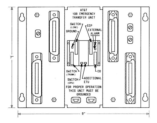
Figure 2-31. 10B Emergency Transfer Unit (ETU)
