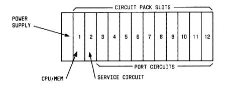
a) CABINET 1 - (MOUNTING FOR CONTROL & PORT CIRCUIT PACKS)
