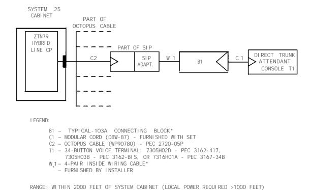
Figure 2-2. Direct Trunk Attendant Console Connections
