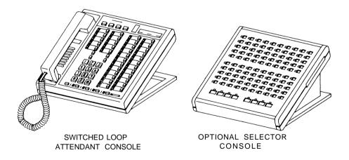
Figure 2-3. Typical Switched Loop Attendant Console Position
