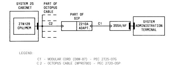
Figure 2-50. SAT On-Premises Direct Connections (Sharing Same AC Outlet)
