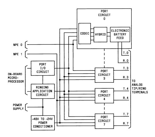
Figure 3-17. Tip Ring Line (ZTN78) Unique Circuitry
