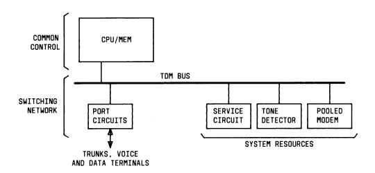
Figure 3-1. System 25 Digital Switch
