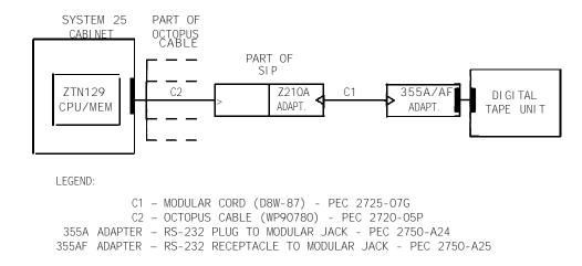
Figure 2-17. Digital Tape Unit—On-Premises Direct Connections (Sharing Same AC Outlet)
