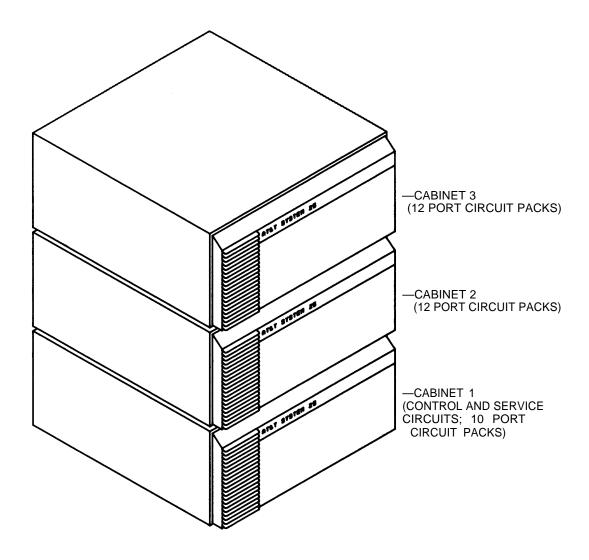
Figure 4-1. System 25 Cabinets (J58901A)—3-Cabinet System
