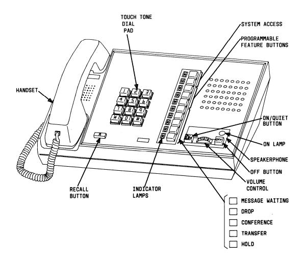
Figure 4-20. 10-Button MET With Built-In Speakerphone (2993C04)
