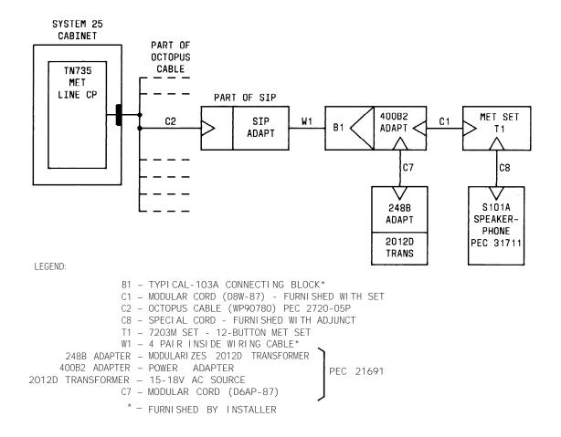
Figure 2-37. Speakerphone Connections For 12-Button MET Sets
