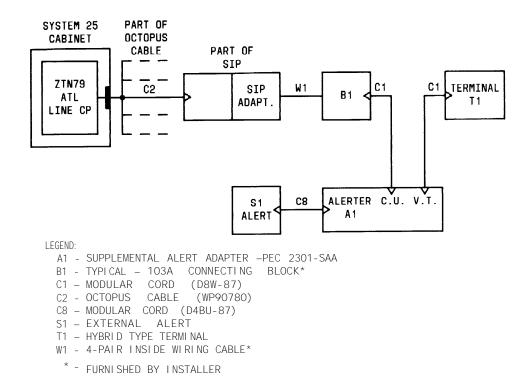
Figure 2-20. Supplemental Alert Adapter Connections
