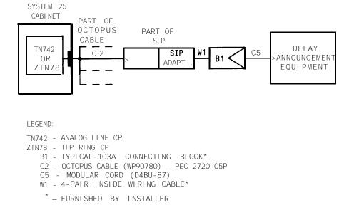
Figure 2-18. Delay Announcement Equipment Connections (FCC Registered)
