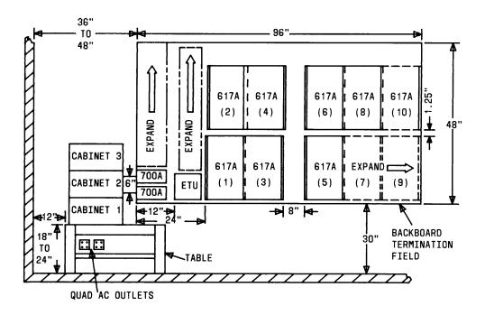
Figure 6-2. Typical System 25 Equipment Area Elevation Plan
