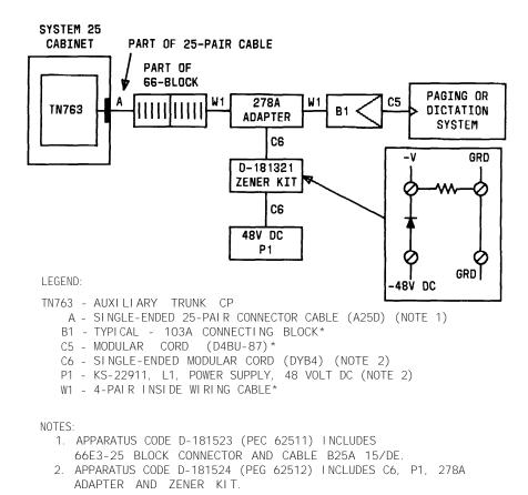
Figure 2-30. Paging Equipment Connection to TN763 Causing 278A Adapter
