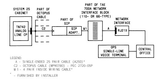
Figure 4-28. Off-Premises Station Single-Line Voice Terminal Connections
