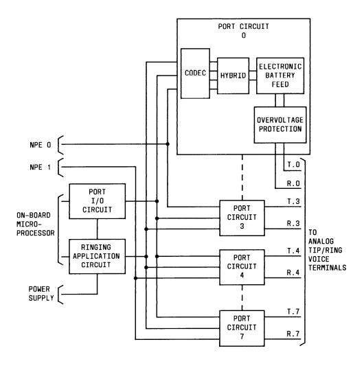
Figure 3-7. Analog Line (TN742) Unique Circuitry
