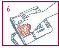
Attach the receiver card and lens (shiny-side down).
