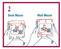
Attach the wedge-shaped base in desk mount or wall mount<sup>†</sup> position.
