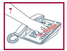
Attach the memory key card and lens (after saving numbers and names in memory). The lens snaps on and off so you can add numbers.
