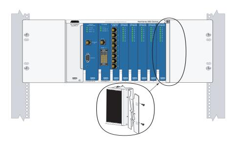
Figure 11. Rack Mounting the NetVanta 950 IAD
