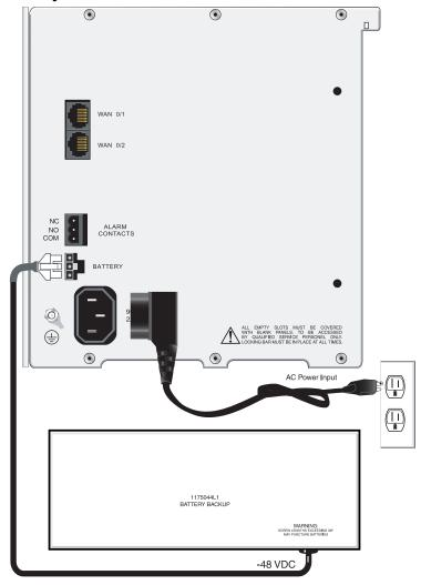
Figure 12. NetVanta 950 Battery Pack Connections
