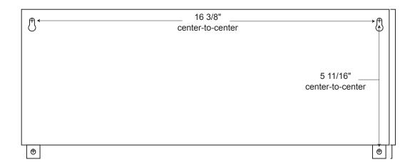
Figure 13. Battery Pack Mounting Dimensions
