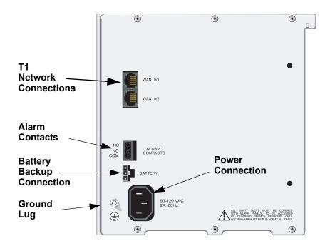
Figure 3. NetVanta 950 Left Side Panel Layout
