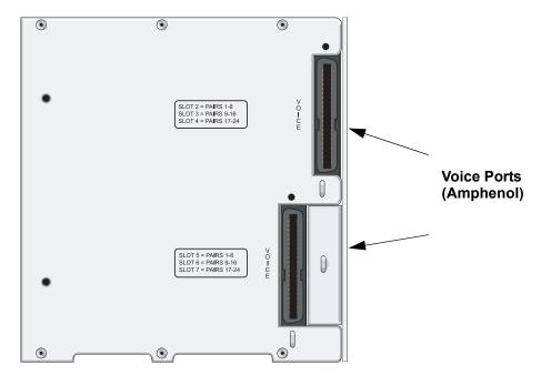
Figure 2. NetVanta 950 Right Side Panel Layout
