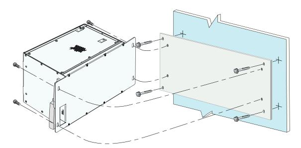
Figure 10. Wallmounting the NetVanta 950
