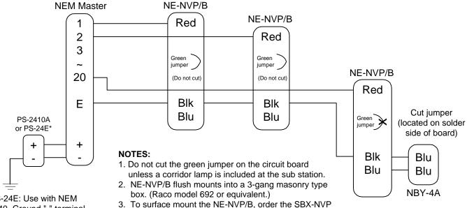
\*PS-24E: Use with NEM 30/40. Ground "-" terminal to earth ground, not "Gnd" terminal.
