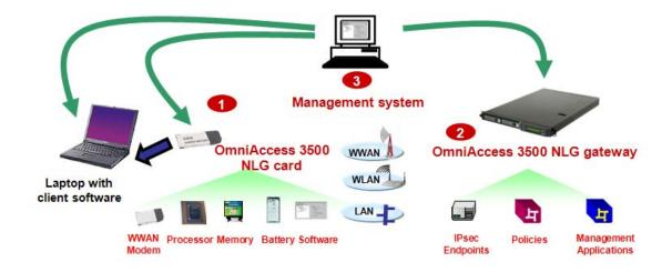
Figure 1 displays the OmniAccess 3500 NLG platform components.
