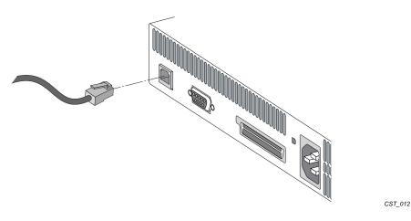
Connect the serial console port using an RS-232 cable with a DB-9 connector, as shown in *Figure 15*. The default settings for this port are 9600 baud, 8 data bits, 1 stop bit, and no parity or flow control (9600 8-N-1 none). The default settings may be changed either in the boot monitor or during system operation.
