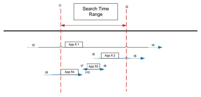
*Figure 59* shows that a search for an active application "*App*" between t1 and t2 time period results in a sum of bandwidth (bytes, packets) of all the application flows (*fl1* – *fl4*). The start time of the application comes up as t3 and the last occurrence time shows up as t4.
