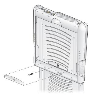
FIGURE 7 Removing the Label
