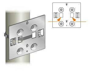
FIGURE 5 Mounting the Cradle to a Vertical Post
