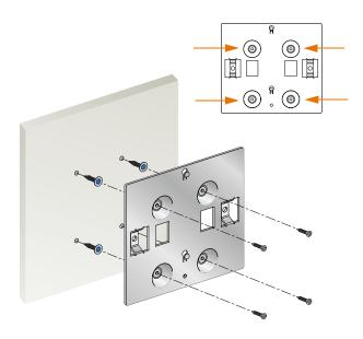
FIGURE 2 Attaching the Cradle to a Solid Surface
