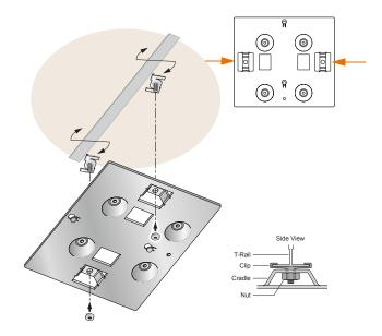
FIGURE 4 Mounting the Cradle to a Suspended Ceiling
