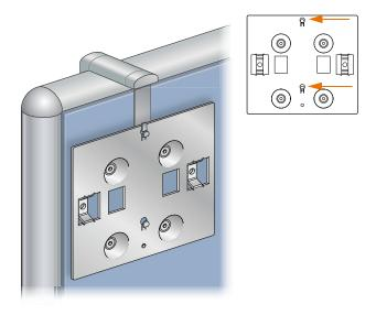
FIGURE 6 Mounting the Cradle to a Partition Hanger
