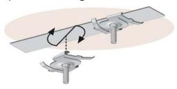
FIGURE 3 Attaching the T-Rail Clips
