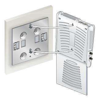
FIGURE 8 Placing the A70 into the Cradle
