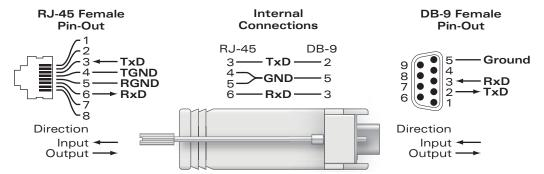
FIGURE B-5 Serial Port Adapter
