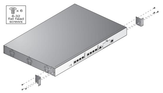
FIGURE 2-2 Attaching the Rack Mounting Brackets
