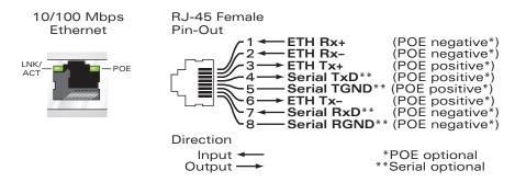
FIGURE B-2 FE Network Port Pin-outs
