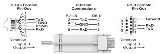
FIGURE B-5 Serial Port Adapter
