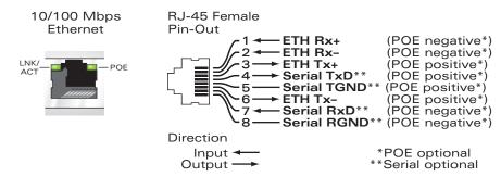
FIGURE B-2 FE Network Port Pin-outs
