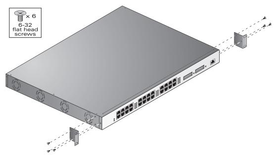
FIGURE 2-2 Attaching the Rack Mounting Brackets
