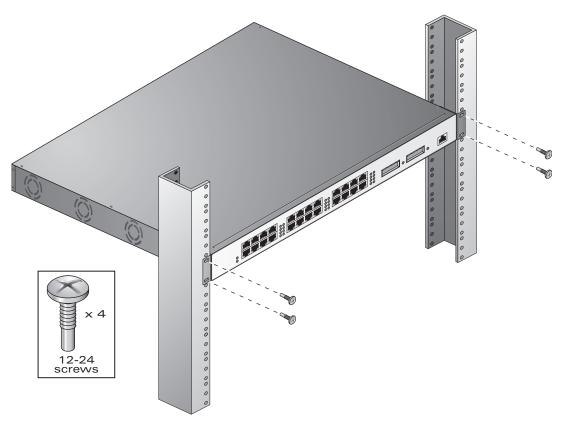
FIGURE 2-3 Mounting the Alcatel Wireless LAN Switch
