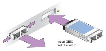
Squeeze Release Tabs and Remove GBIC
