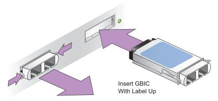
Squeeze Release Tabs and Remove GBIC
