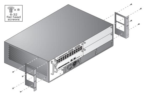
FIGURE 2-2 Attaching the Rack Mounting Brackets
