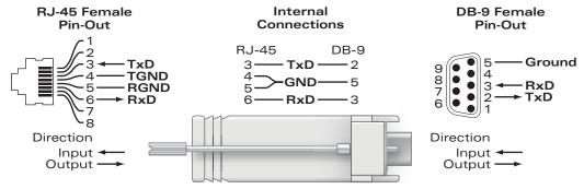
FIGURE 6-3 Serial Port Adapter
