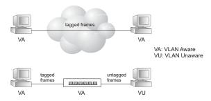
Figure 3-70. Tagged and Untagged Frames
