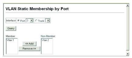
Figure 3-77. VLAN Static Membership by Port
