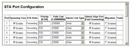
Figure 3-66. STA Port Configuration
