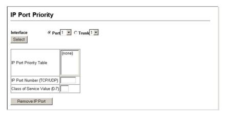
Figure 3-14. Mapping Switch Ports and Trunks to IP TCP/UDP Priority
