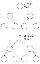
to those ports only. It then propagates the service request up to any neighboring multicast switch/router to ensure that it will continue to receive the multicast service. This procedure is called multicast filtering.
