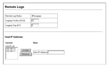
Figure 3-5. Enabling Remote Logging and Adding Host IP Addresses
