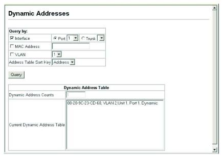
Figure 3-59. Setting a Dynamic Address Table
