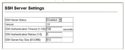
Figure 3-25. Secure Shell Server Settings
