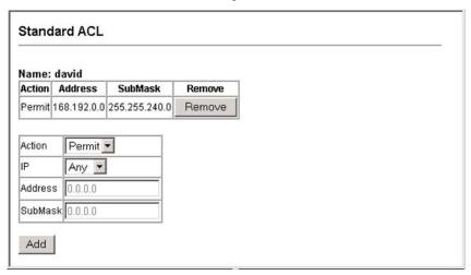
Figure 3-33. Configuring a Standard ACL
