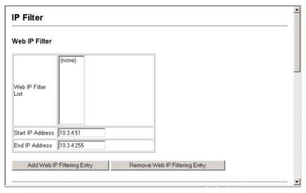
Figure 3-12. Filtering IP Addresses
