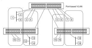
Figure 3-71. Port Based VLANs
