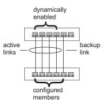
**Web** – Click Port, LACP, Configuration. Select any of the switch ports from the scroll-down port list and click Add. After you have completed adding ports to the member list, click Apply.
