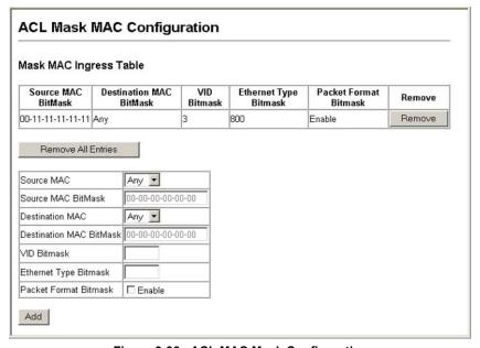
Figure 3-38. ACL MAC Mask Configuration
