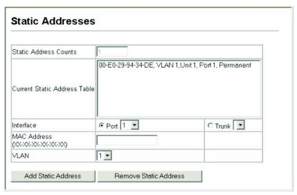
Figure 3-58. Setting a Static Address Table
