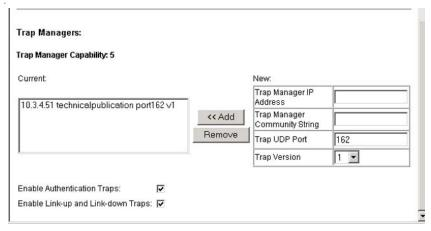
Figure 3-19. Configuring SNMP Trap Managers
