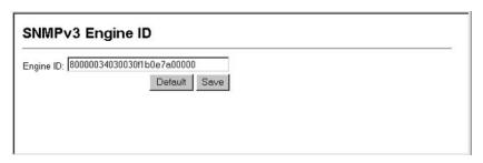
Figure 3-8. Setting an Engine ID
