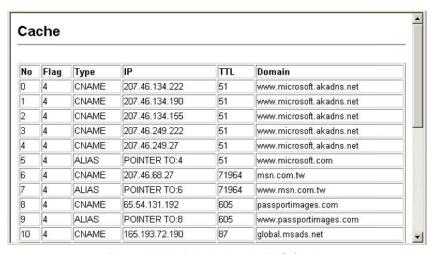
Figure 3-108. Displaying the DNS Cache
