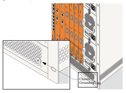
**Important.** For the grounding wrist strap to be effective in eliminating ESD, power supplies must be installed in the chassis and plugged into grounded AC outlets.
