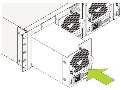
**4** Continue sliding the power supply back until the front panel meets the front of the chassis. *Do not force the power supply into the bay. Otherwise you can damage the connectors.*
