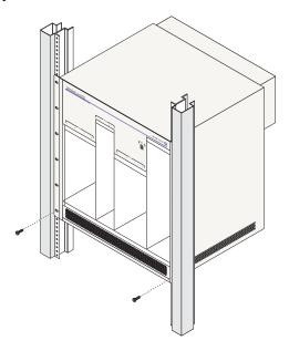
**Note.** Be sure to install the screws in the *bottom hole* of each flange, as shown, before proceeding.
