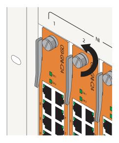
**2** Next, simultaneously pull the two module extractor levers—one on top of the module and one on the bottom—until the module disengages from the chassis.
