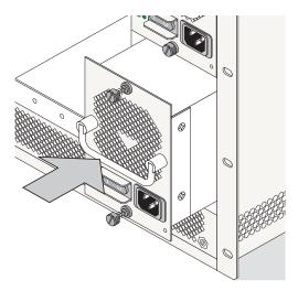
**5** Continue sliding the power supply back until the front panel meets the front of the chassis. *Do not force the power supply into the bay. Otherwise you can damage the connectors.*
