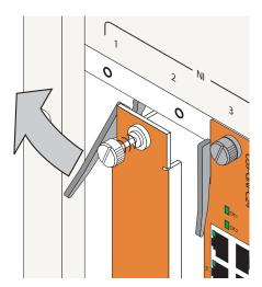
**3** Holding the module in both hands, carefully slide it out of the chassis along the card guide. The module should slide out easily. Do not force the module from the slot.
