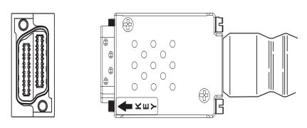
**Important.** Please note the "KEY" label on the connector. One side of the connector has a curve to it and the other side is straight. Therefore, to correctly orient the cable, make sure that the "KEY" label is at the top.
