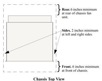
**Note.** Never obstruct the air intake vents located at the bottom-front and bottom-sides of the chassis *or* the fan unit's air output vents located at the rear of the chassis. Clearance is not required at the top and bottom of the chassis.
