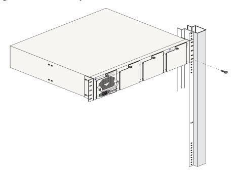
**Note.** Be sure to install the screws in the *bottom hole* of each flange, as shown, before proceeding.
