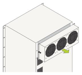
Detach the fan tray by pulling it straight out and away from the chassis.
