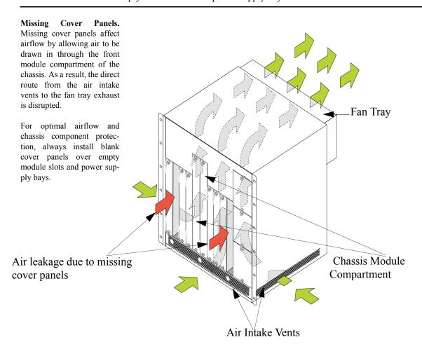
**Effects of Missing Blank Panels on Chassis Airflow**
