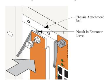
**4** Once the module is firmly seated, secure the module to the chassis by tightening the two captive screws. *Be sure not to overtighten the captive screws. If you use a screwdriver, the torque used to tighten the screws must not exceed 2.3 foot-pounds.*
