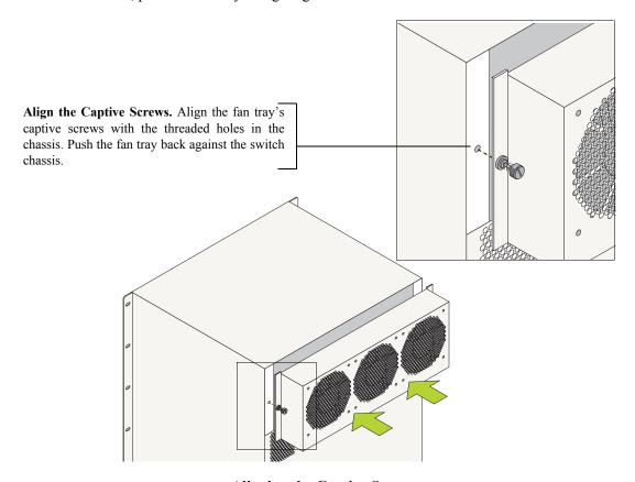
**Aligning the Captive Screws**
