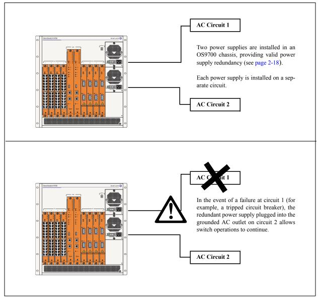
**OS9700 Redundant AC Circuit Example**
