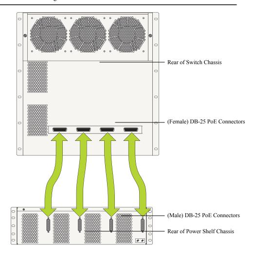
**Important.** The connectors on the rear of the switch chassis and the power shelf chassis are for PoE power connections only. *Never attempt to connect data communication or other equipment to these connectors*.
