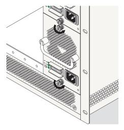
**4** With one hand, grasp the handle at the front of the power supply and slowly pull the power supply out of the power supply bay. *Do not pull the power supply completely out of the bay with one hand.*
