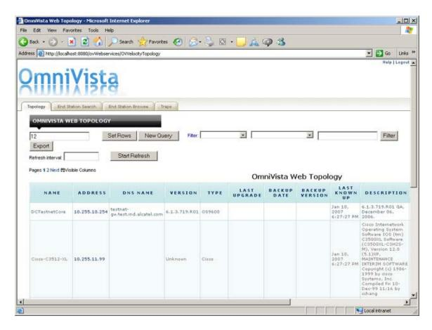
The Web Client Topology screen provides a listing and description of all discovered switches. From here, you can perform OmniVista Topology functions. You can also click on the End Station Search or End Station Browse tabs to access Locator functions; or click on the Traps tab to access Notifications Functions.
