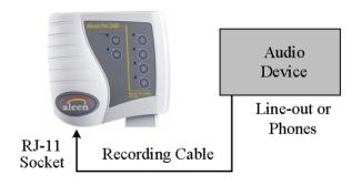
Figure 3-1. Connecting the Recording Cable
