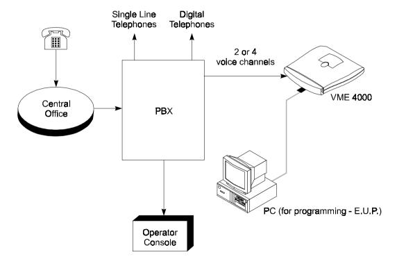
Figure 2-6 System Installation
