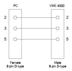
Figure 4-1 RS-232 Cable Connection
