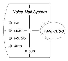
Figure 2-4 LEDs on the Front Panel
