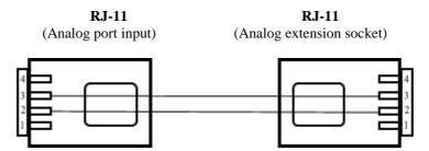
Figure 2-2: Analog Ports Input Cable
