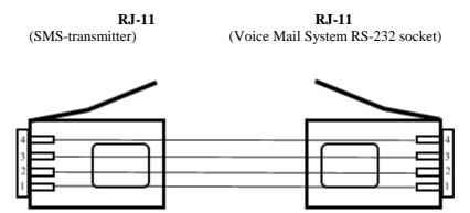
Figure 8-3: SMS Transmitter Communication Cable
