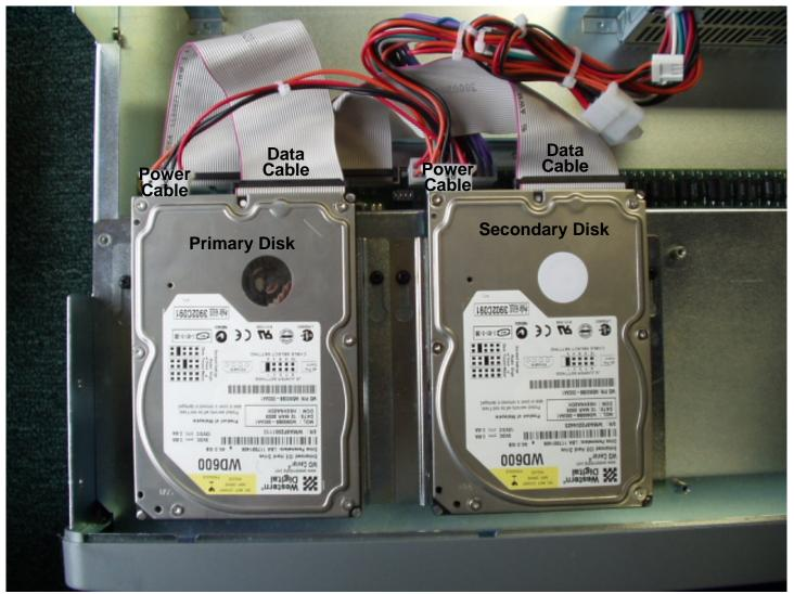
Figure 4 - Disk Positions and Cabling
