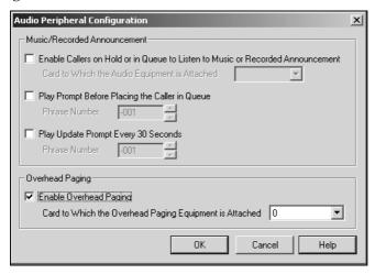
Figure 54. Audio Peripheral Configuration window
