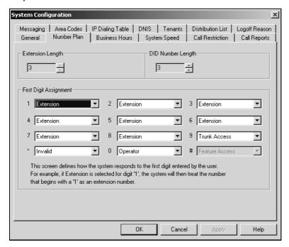
Figure 2. Number Plan window, System Configuration
