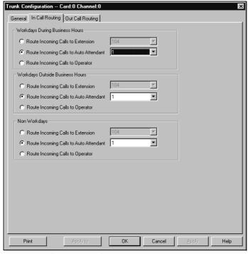
Figure 31. In Call Routing window, Trunk Configuration
