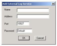
Figure 4. Enable external RTM data logging
