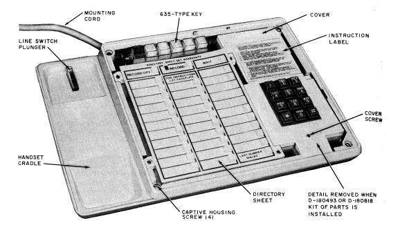
Fig. 2—2872A2M Telephone Set—Faceplate and Handset Removed
