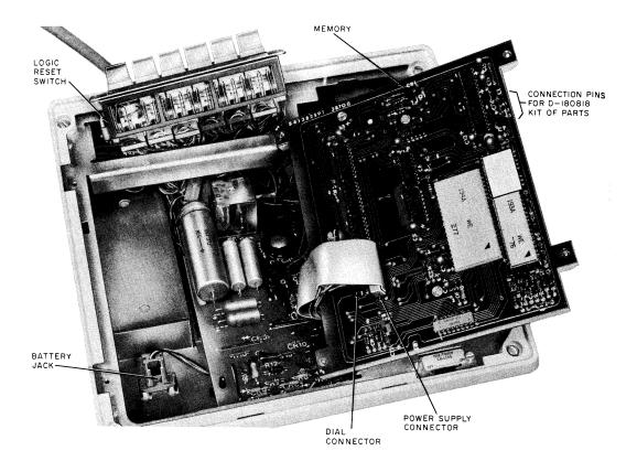
Fig. 5—2872A2M Telephone Set, Internal View, Overall
