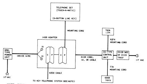
NOTE: DISCONNECT THE (V-BL) AND (BL-V) LEADS IN THE CABLE AT KEY SYSTEM END
