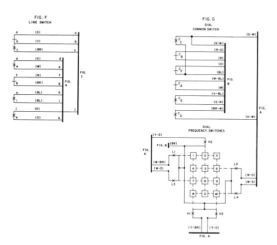
Fig. 9—2872A1M (MD) or 2872A2M Telephone Set, Connections (Sheet 3 of 5)
