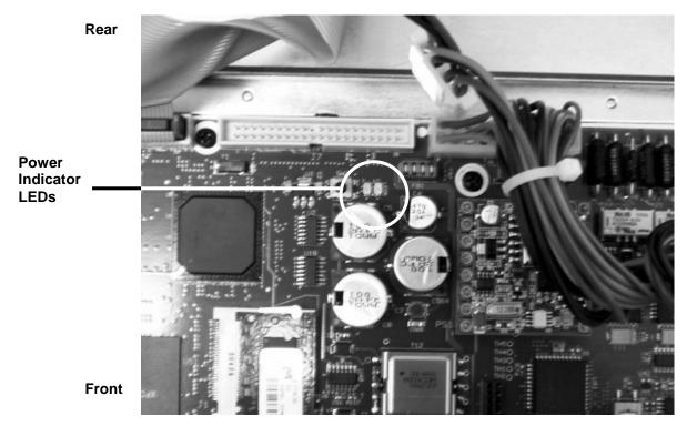
Figure 3: Motherboard Power Indicator LEDs
