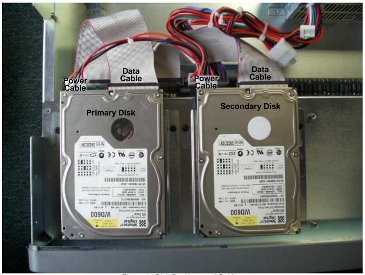
Figure 4 - Disk Positions and Cabling
