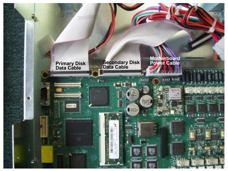
Figure 5 - Motherboard Disk and Power Cables
