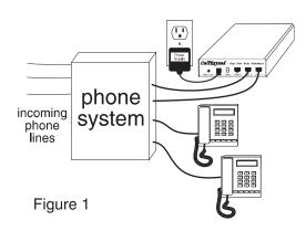
**Note:** Typically, if both ports of CallExtend are to be used, incoming calls should be routed first to the phone system extension that is connected to CallExtend's Port 1. Calls should then hunt to the phone system extension connected to CallExtend's Port 2. Do **not** have each incoming call ring simultaneously to both of the phone system extensions that CallExtend is connected to.
