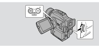
Immediately after you have recorded a still image to a memory card, you can check the image without switching the operation mode by the POWER switch. (CARD PHOTO REVIEW)
