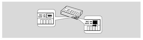
To protect your recording from accidental erasure, slide the tab on the cassette so that it exposes the hole. (This switch position is usually labeled SAVE or ERASE OFF.)
