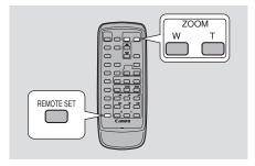
The wireless controller and the camcorder have been preset to mode 1. If you change the mode on the camcorder, be sure to change the mode on the wireless controller to the same mode.
