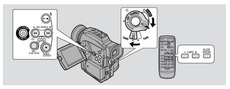
Play back and view still images recorded on a memory card. (For details on connecting to a TV, see "Connections for Playback on a TV Screen" on p. 32)
