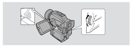
Adjust the speaker volume by turning the selector dial.
