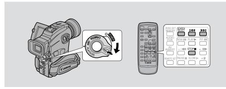
This allows you to move quickly through still pictures recorded anywhere on a tape (photo search) or between different days or areas of recording (date search) on a tape.
