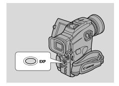
To lock the exposure, press the EXP button. Press it again to return to auto exposure.
