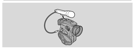
For greater creative control over audio recording, you can connect an external microphone to the camcorder via the MIC terminal. When using the MIC terminal, use a microphone with a built-in power supply (condenser microphone). It is possible to connect almost any stereo microphone with a plug diameter of ½ inch (3.5 mm), however, their audio levels will be different from that of the built-in microphone.
