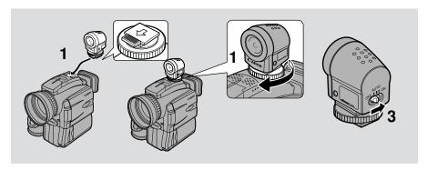
When recording in dark rooms, attach the Video Light to the camcorder's "S" advanced accessory shoe. The Video Light is powered by the same power source as the camcorder.
