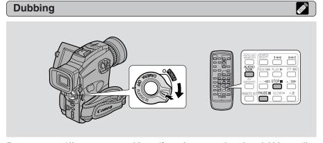
Do not connect/disconnect any cables to/from the camcorder when dubbing audio or preparing to dub audio.
