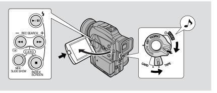
You can use the LCD screen for instant, on-the-spot playback. When using the LCD screen, the camcorder also plays back the sound track via the built-in speaker ( \sum 31).
