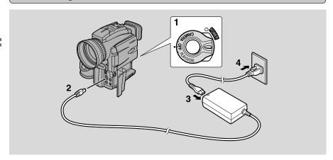
Use the power adapter to provide your camcorder with instant power from an AC outlet. Always turn the camcorder off before connecting/removing the power source.
