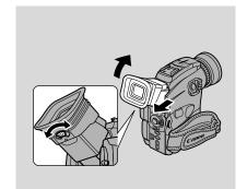
Be careful not to leave the viewfinder exposed to bright sunlight, or it will melt. (The light is concentrated by the viewfinder lens.) Adjust the angle of the viewfinder to prevent sunlight from entering.
