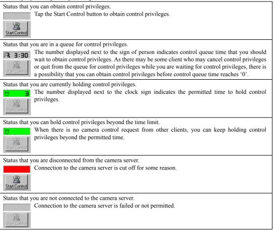
It is not guaranteed that control privileges can be obtained immediately whenever you wish. Note Check the camera control status before you try to control the camera.
