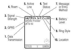
**1. Data Transmission Indicator** Shows connection and data transmission status. Indicators can include:
