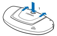
2 To remove the front cover, gently pull the cover on both sides (1) and remove the cover starting from the top (2).
