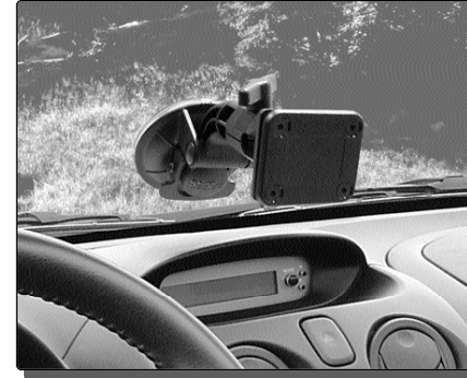
The suction cup portion of the bracket can be left attached to the windshield for quick reinstallation.
