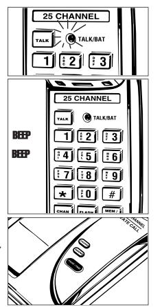
The rechargeable NiCad battery in your cordless phone may need to be replaced if the handset will not function when the TALK button is pressed after recharging for 12 hours.
