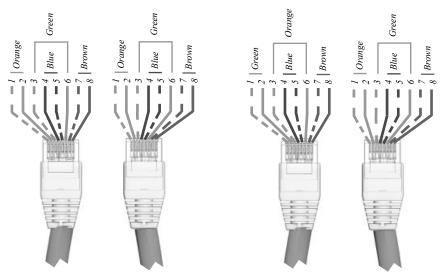
*Straight through cable: Notice how both ends are identical*
