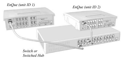
Make sure a computer is connected to the phone system either via the LAN or directly from the computer to the EnQue through the USB or Serial port.
