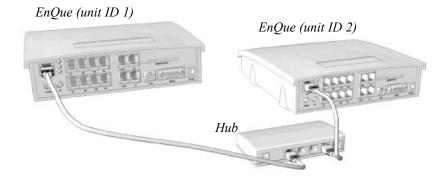
Connect up to four EnQue units (2 are shown here) to the LAN hub. Make sure a computer is connected to the phone system either via the LAN or directly from the computer to the EnQue through the USB or Serial port.
