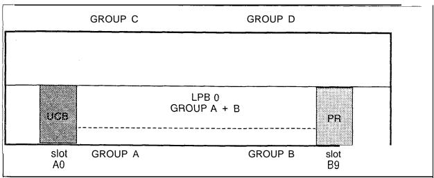
Figure 12.1 Example of Single Local Packet Buses in Groups A & B
