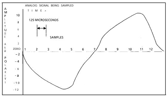
Figure 4.8 Sampling an Analog Signal
