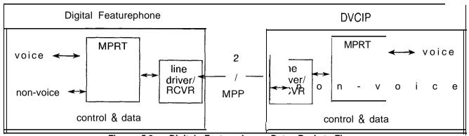
Figure 5.8 Digital Featurephone Data Packet Flow
