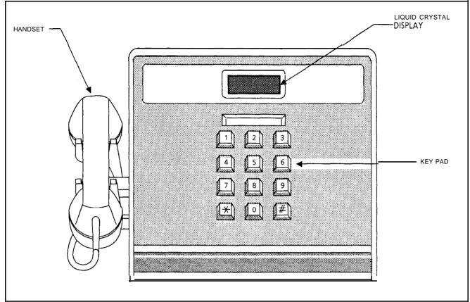
Figure 17.1 Display Telephone
