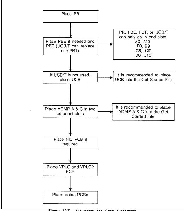
Figure 12.7 Flowchart for Card Placement
