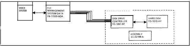
Figure 4.14 FMSD and Hard Disk Assembly Interface
