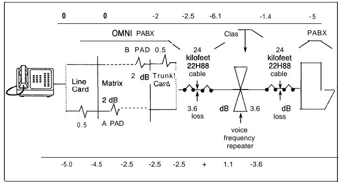
Figure 36.4 Line to Nontandem I is I runk Call (VNLP)
