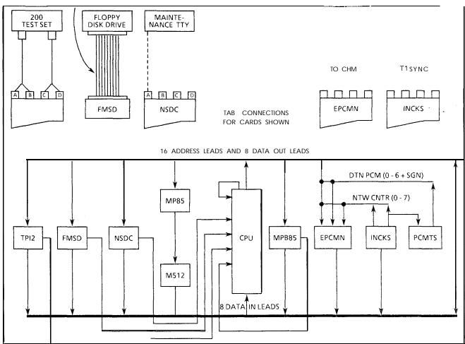
Figure 4.1 CPU Connections
