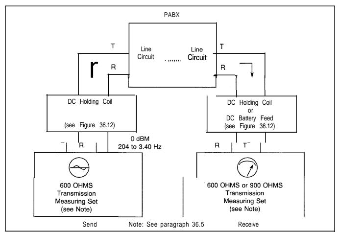
Figure 36.13 Insertion Loss and Frequency Response Measurement
