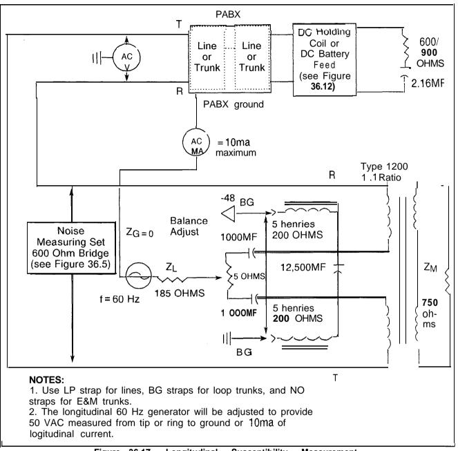
Figure 36.17 Longitudinal Susceptibility Measurement
