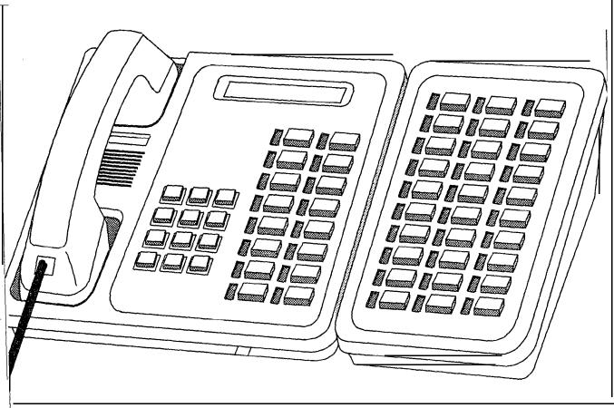
Figure 3.1 Featurephone With 30-Button Add-On Module
