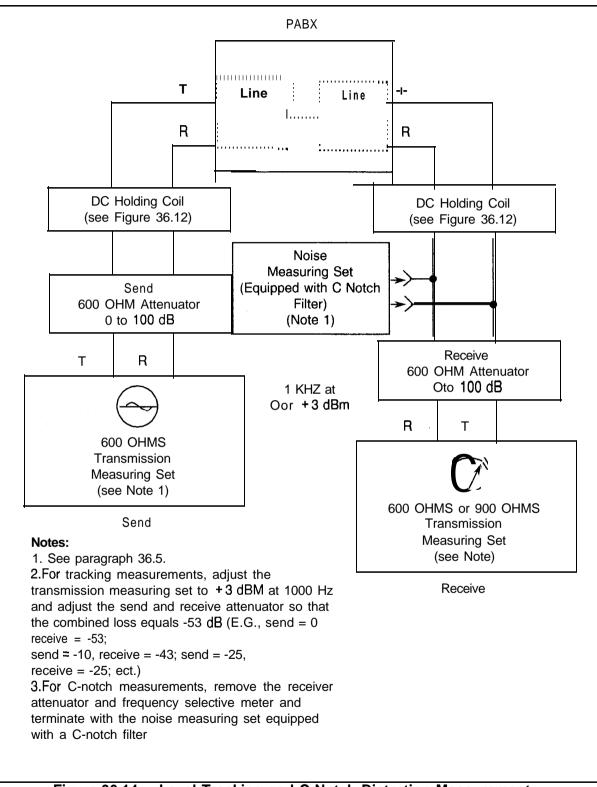
Figure 36.14 Level Tracking and C-Notch Distortion Measurement
