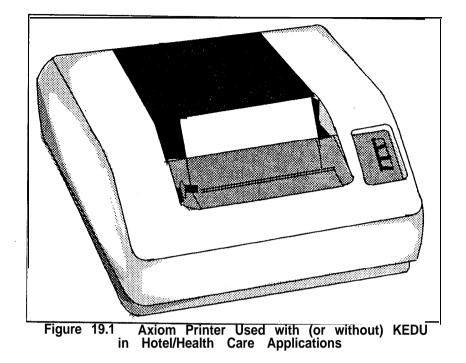
H/HC Printer/System Interface **19.1** The **printer interfaces** with the system via the SIDML card, located in a PCMUS slot.
