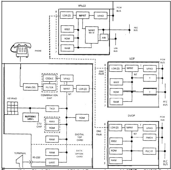
Figure 17.4 Block Diagram of Digital Featurephone with VCIP or DVCIP Card
