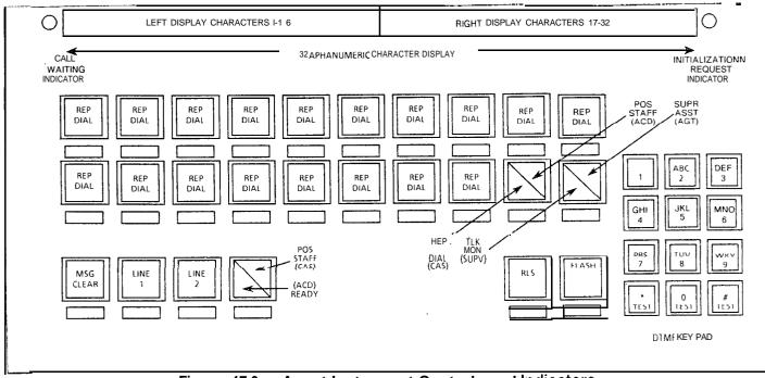
Figure 17.6 Agent Instrument Controls and Indicators
