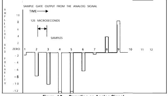
Figure 4.7 Sampling an Analog Signal
