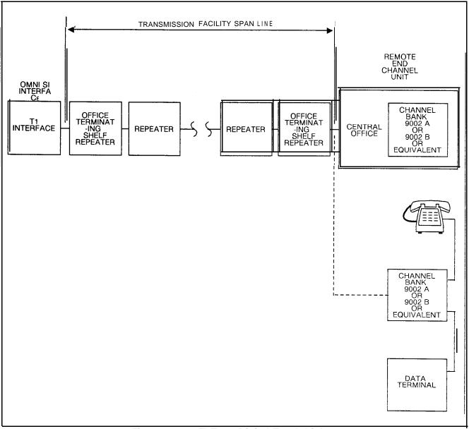
Figure 29.1 TI-Type Digital Trunk Link
