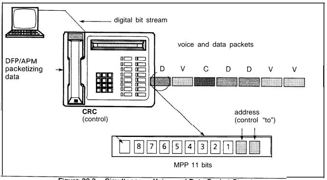
Figure 33.3 Simultaneous Voice and Data Packet Structure
