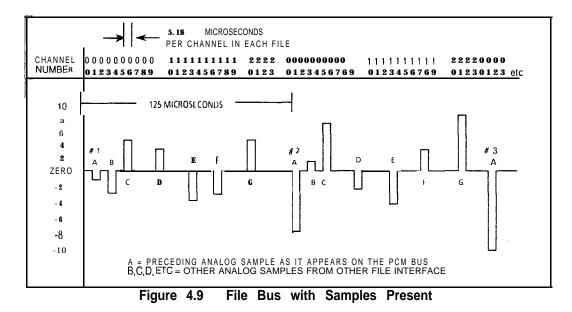
All time-switch network functions must be performed for each active circuit in only 0.000000648 second. Conversely, the network performs 1,544,000 time slot processes every second. Each time slot process is performed in four different time intervals or periods (called cycles) within this 648 nanosecond period, which means a 162 nanosecond cycle period or a 6.17 MHz rate. Figure 4.10 shows the time-switch network and PCMUS group interleaving.
