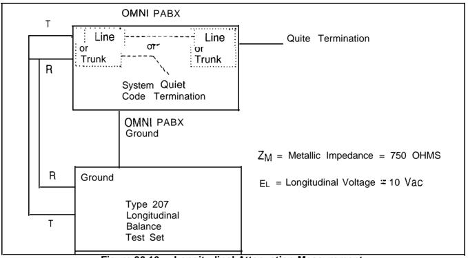
Figure 36.16 Longitudinal Attenuation Measurement
