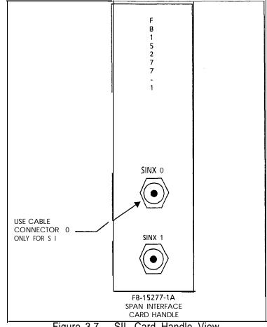
NOTE: To synchronize the PABX digital network timing to the T1 -span timing, use FB-15277-I.
