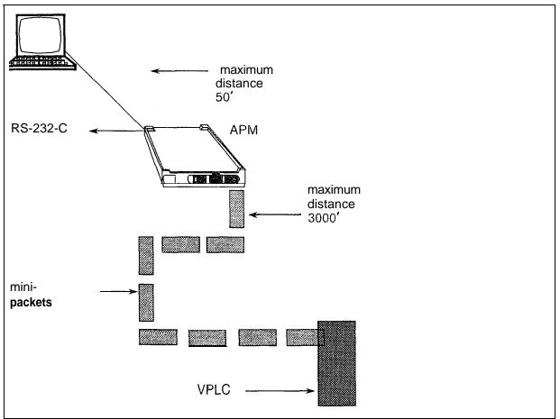
Figure 31.3 Transport of Mini-Packets
