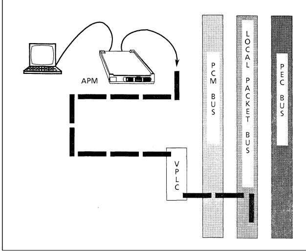
Figure 8.5 Transportation of Mini-Packets over LPB
