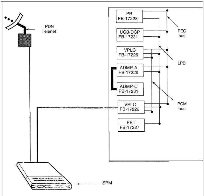
Figure 32.2 Synchronous Packet Manager Interface
