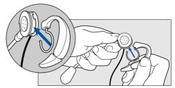
Figure 6 Installing Ear Capsule
