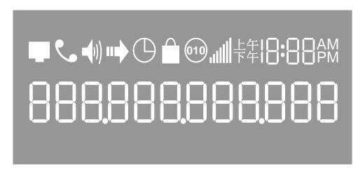
When the phone is in the normal idle state, the backlight is off. Whenever an event (call) occurs, the backlight and the red LED will turn on automatically to bring the user's attention. In addition, if Voice Mail configured and there is a VM waiting, the backlight will be blinking and the red LED message light will light up to remind user there is a Voice Mail in the Voice Mail server.
