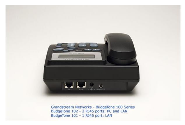
The ONLY difference between BT101 and BT102 is that the two RJ-45 ports of BT102 is actually a 10Base-T **mini-Hub** that allows user to share or sniffer the network using another data device like PC.
