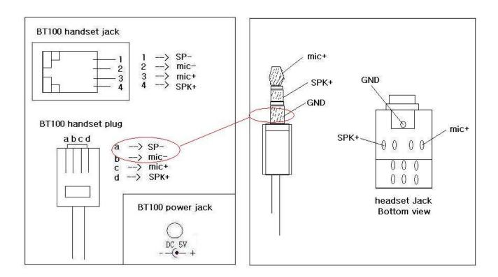
The picture below shows the handset and headset connectors' wiring schema.
