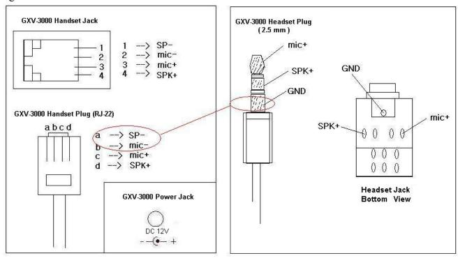
As show in the schema, the left side is pin assignment of a RJ-22 handset plug; while the right side is showing a normal 2.5mm headset plug. If use want to connect the phone to external Speaker or Intercom/Paging system, necessary adaptors are required from local electronic stores.
