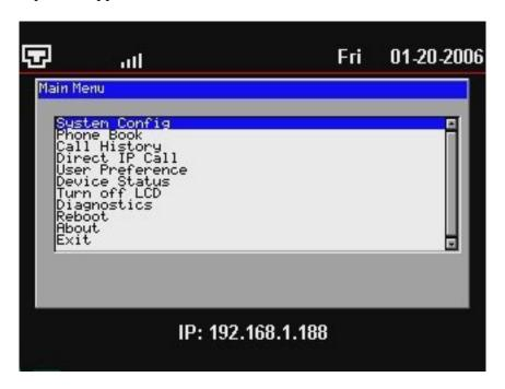
Here is the flow chart of keypad Menu configuration. During operation of the keypad, OK key is function as select or confirm key (similar to Enter in PC), UP and DOWN arrow keys are functioning as browsing (by highlight the item selected), LEFT and RIGHT arrow keys are functioning as input selection, MUTE/DEL key is functioning as delete if input is wrong.
