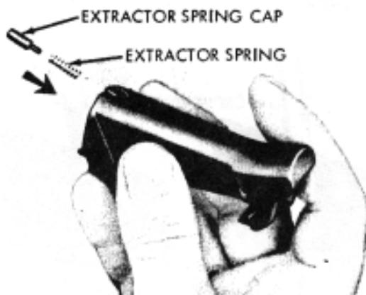
5. Install positive extractor spring and positive extractor spring cap.
