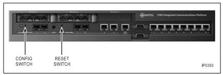
Figure 14: CONFIG and RESET switches
