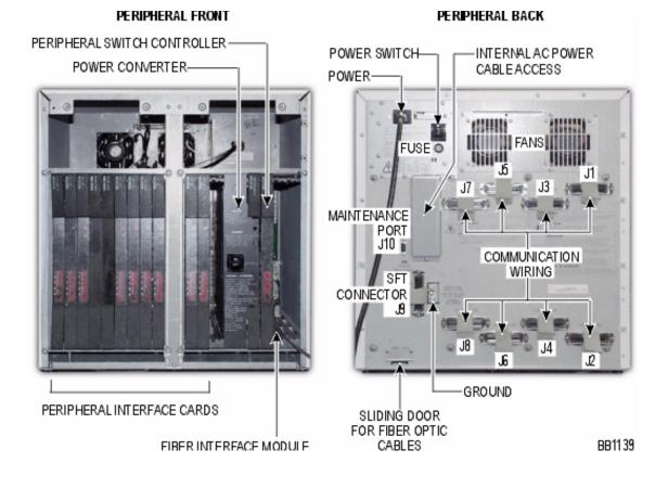
The peripheral cabinet consists of the following components:
