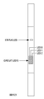
One status LED and fifteen circuit LEDs are mounted on the faceplate. The status LED shows the status of the CEPT link, and each of the circuit LEDs shows the status of one BRI circuit. The BRI circuit LEDs are also used during card initialization to indicate the progress of the self-test and to indicate that the download is in progress.
