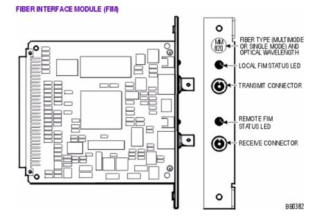
There are two LEDs on each FIM. The top LED indicates the status of the FIM itself; the bottom LED indicates the status of the other FIM (the FIM connected to the far end of the fiber optic cable).
