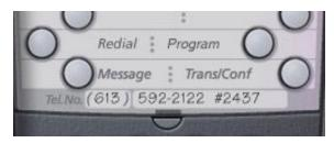
Note: The three bottom-most programmable function keys should be labelled REDIAL, MESSAGE and TRANS/CONF. The top-left programmable function key will automatically be assigned as the primary LINE key.
