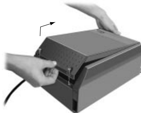
Figure 1-1 REMOVING THE 28i COVER
